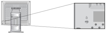
Figure 2. Kensington-type security slot location
